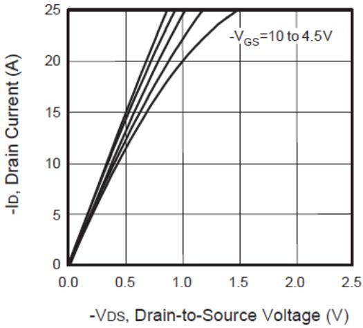
Figure 1. Output Characteristics
