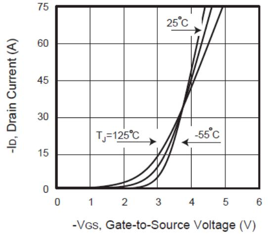
Figure 2. Transfer Characteristics
